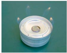
The top/base is used as an insulated support for the fuel cup. This helps keep a stable temperature in the stove and provides protection under the stove. I now use a soda can for the top/base and cut it down until the stove sits firmly without tipping.
