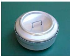
The top/base can be used as a cover for storage or to seal the stove and save fuel between meals. I now use the bottom of a pop can with one 1/16" hole in the bottom- it's lighter and fits tight without getting stuck - no need for the handle. Simmer ring slips over the bottom (not shown in this photo). The package is small enough to store inside of a plastic camp cup.
