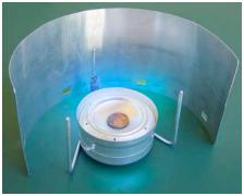
Two "U" shaped wires wrapped together with thin wire form the pot pupport. Drip irrigation stakes work best. Three legs make a stable base- supporting the pot at least 1" above the burner. My windscreen is a section of aluminum Dryer vent. Tests show that screen is not necessary in good weather and only increases one quart boil times by 30 seconds.
